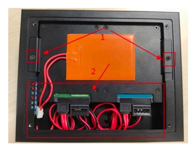
4. Cover the upper cover plate removed from the first step and lock the four screws.
