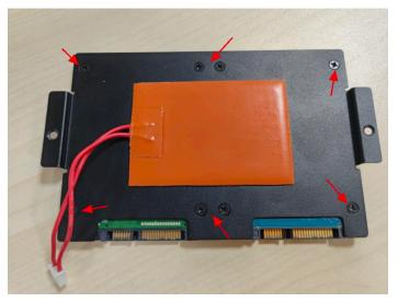
3. Attach the hard drive bracket where the hard drive is installed to the lid of the device, and lock the two screws to secure the hard drive bracket. After that, refer to the screenshot below to connect the hard disk heating cable, SATA power cable, and data cable to the corresponding locations.
