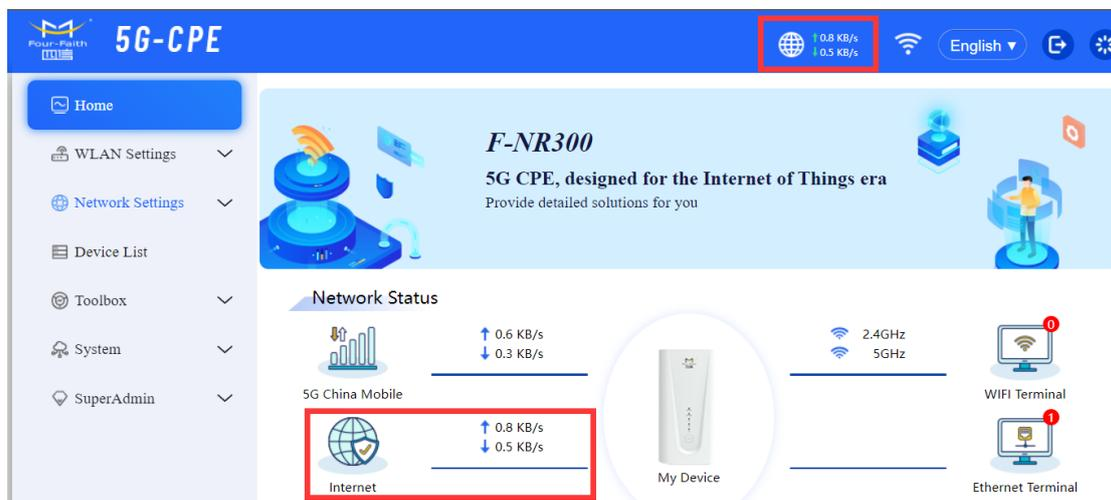
**Step 3:** Connect your terminal device to the CPE's LAN port using an Ethernet cable or connect to the CPE's WiFi network. This will allow your terminal device to access the internet.
