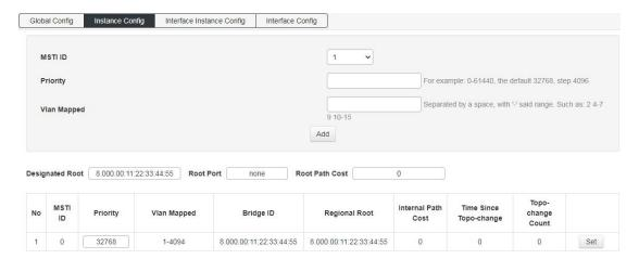
Interface instance configuration: configure the enable of the instance on the port. Screen as blew:
