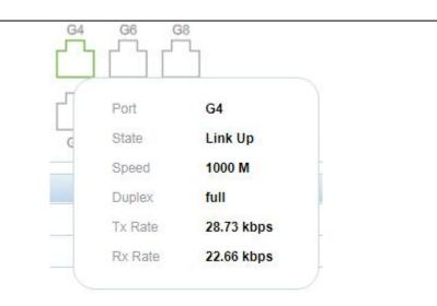
indicates that the port has been enabled and the connection has been established, indicates that the port is not enabled, and indicates the optical port.
