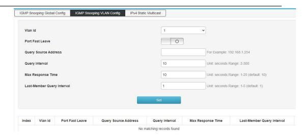
IPv4 Static Multicast: configure static multicast function and enable port static multicast function, screen as blew:
