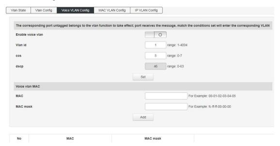
Enable Voice VLAN, the Access port will carry the IP voice traffic from the IP phone. When the switch is connected to Cisco IP phone (such as Cisco 7960 IP phone), the voice traffic sent by IP phone has three layers of IP priority and two layers of CoS value, which are set to 5 by default. For IEEE 802.1Q or IEEE 802.1p tagged traffic, the default cos value is untrusted.
