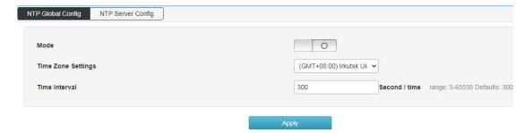
NTP server configuration: configure the NTP server address and view the NTP server status.
