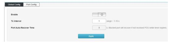
Port Configuration: enable the loop protection function on the port.
