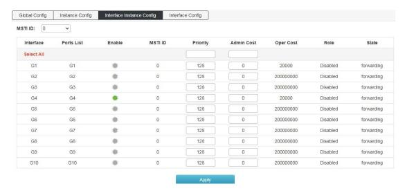
Interface configuration: configure the enabled port of spanning tree protocol and the enabled port of BPDU message. Screen as blew:
