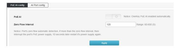
Open the port intelligent power supply function, which is all on by default.
