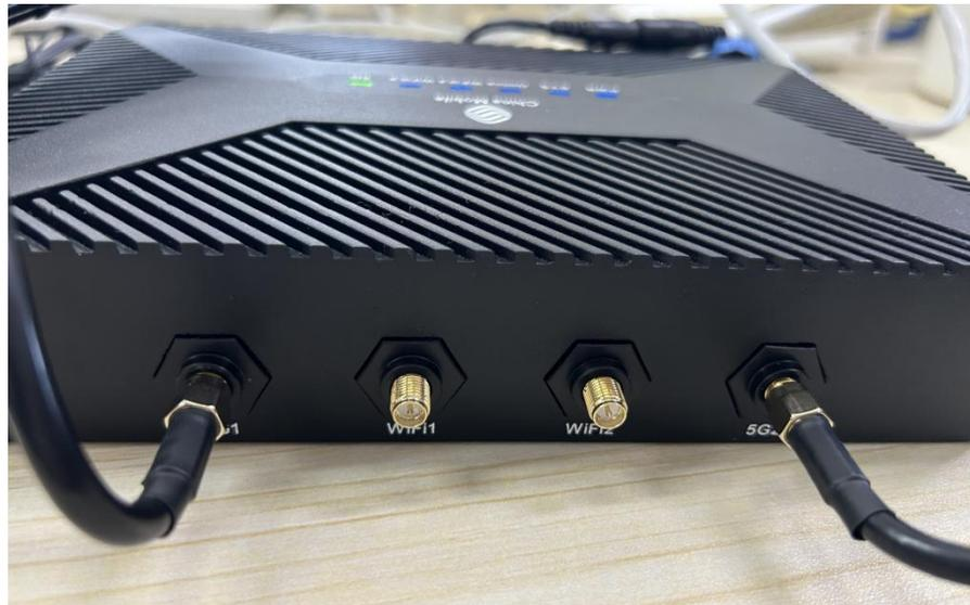
The WIFI antenna interface is an SMA male socket(Identify as "WIFI1" , "WIFI 2" ). Screw the SMA female of the matching WIFI antenna to the antenna interface and make sure to tighten it. In addition, to increase the isolation of the
