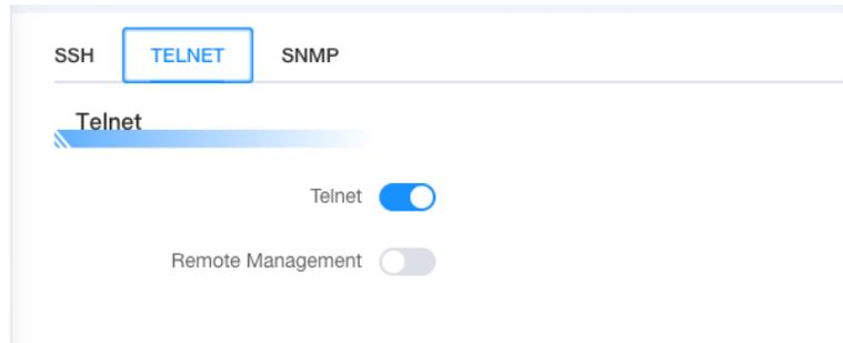
The local Telnet function is enabled by default, and Telnet remote management is disabled by default.
