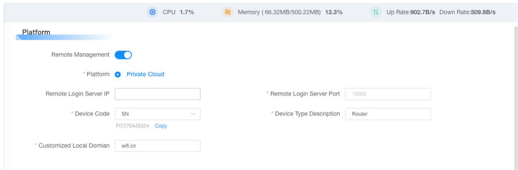
If you have the corresponding device management platform account, you can set the management address of our cloud platform, or if you have subscribed for a private cloud platform deployment, you can set the corresponding cloud platform address and port, and the device code is the SN and unique of the device by default.
