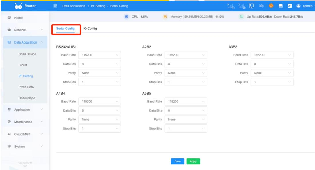
If you do not know the detailed parameters of the docking sub-device, you can perform the following tests, in most serial port equipment, the basic use of 8N1 mode, that is, 8 data bits, 1 stop bit, no verification.
