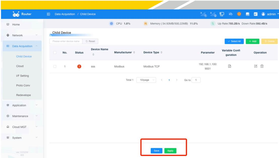
Remember to use the name of the variable in English, because the name here needs to be reported to the MQTT server, and other parameters can be set according to the MODBUS RTU parameters of the device.
