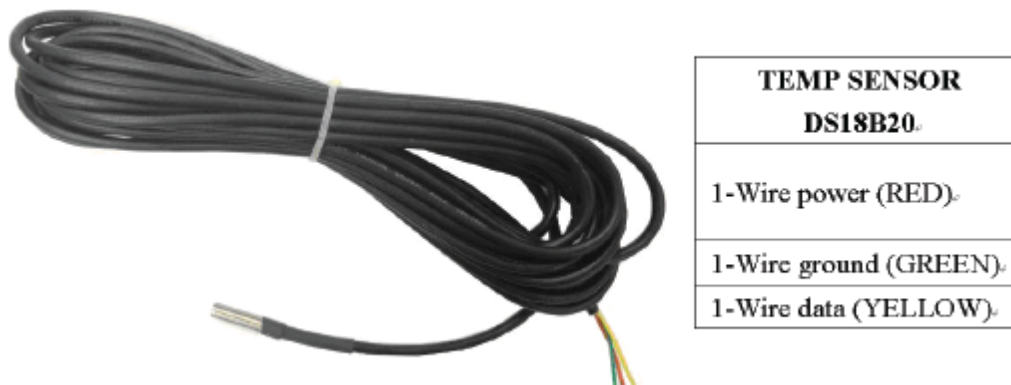
Figure 11: Typical Connection with Temperature Sensor
