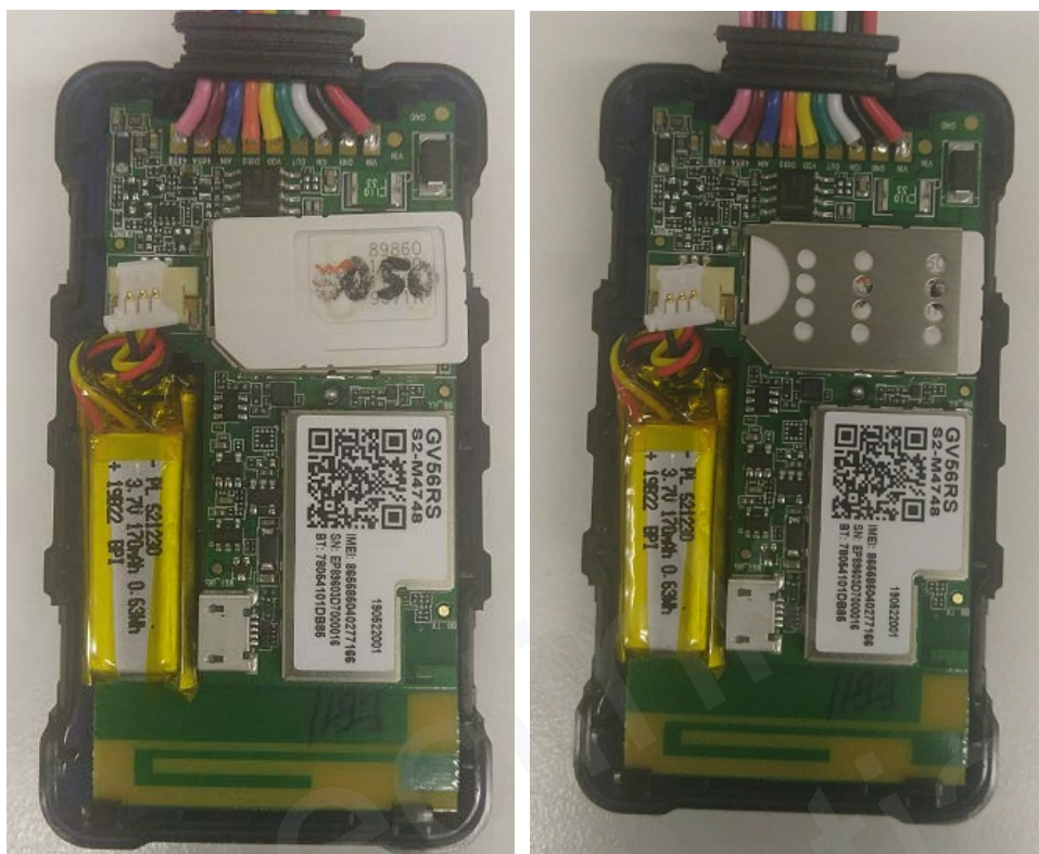
Figure 15: SIM Card Installation
