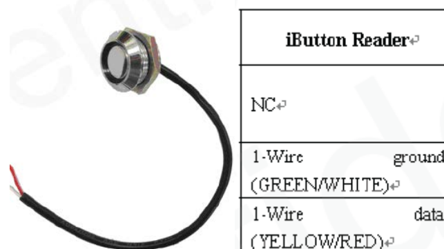
Figure 10: Typical Connection with iButton Reader
