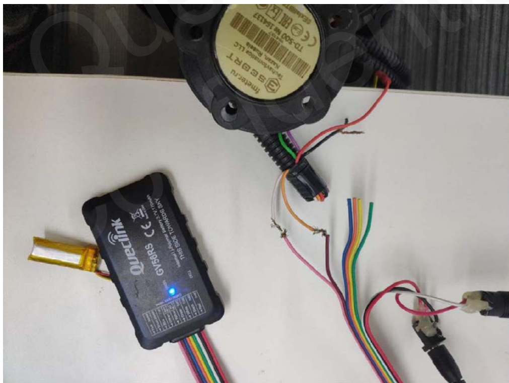
Figure 12: Typical Connection with TD-500 Digital Fuel Sensor
