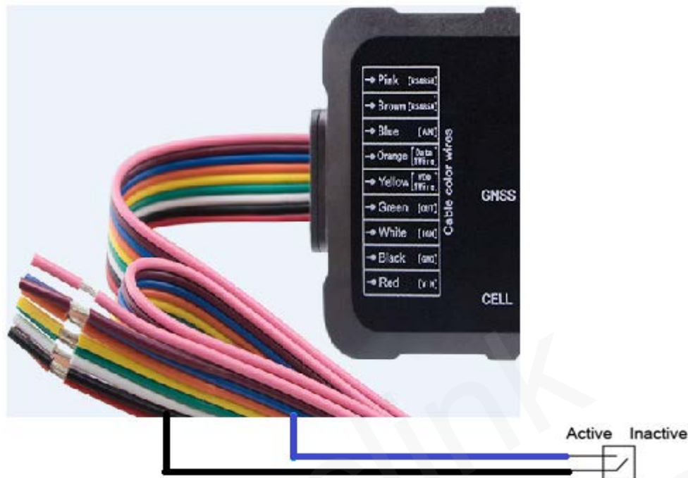
Figure 8: Connection for Negative Trigger Input
