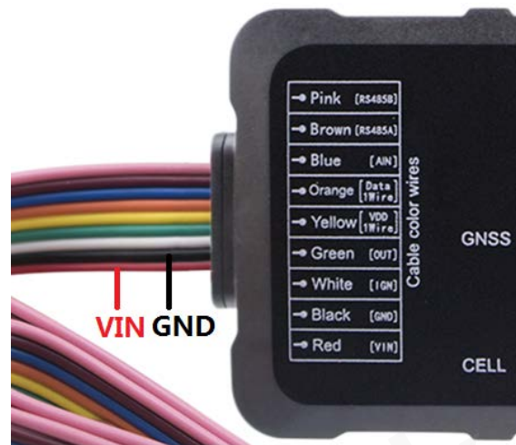
Figure 3: Typical Power Connection
