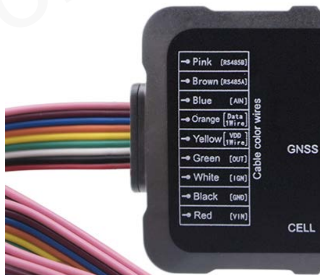
Figure 2: The 9-pin Wire Harness of GV56RS
