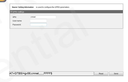
Press the "Send" button and update the parameters of GV56RS. Then GV56RS can report information to your backend server or SMS receiver.
