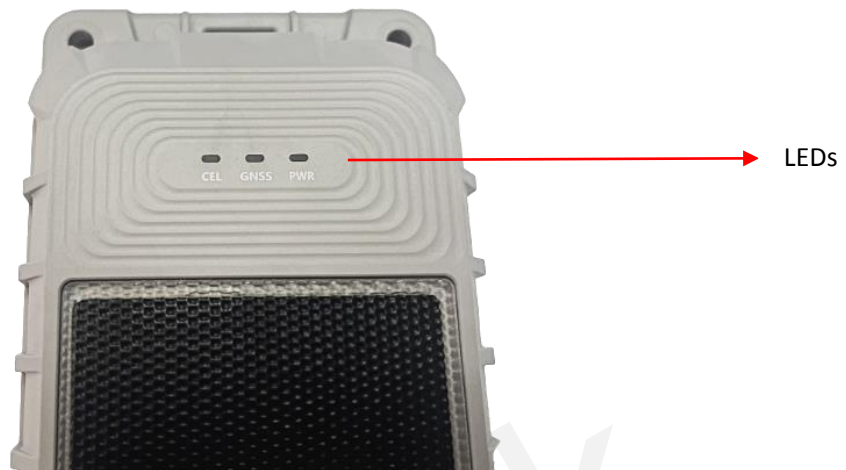
Figure 2. GL601 Series LEDs
