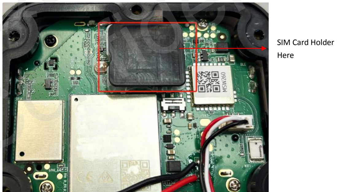
Figure 7. GL601 Series SIM Card Holder
