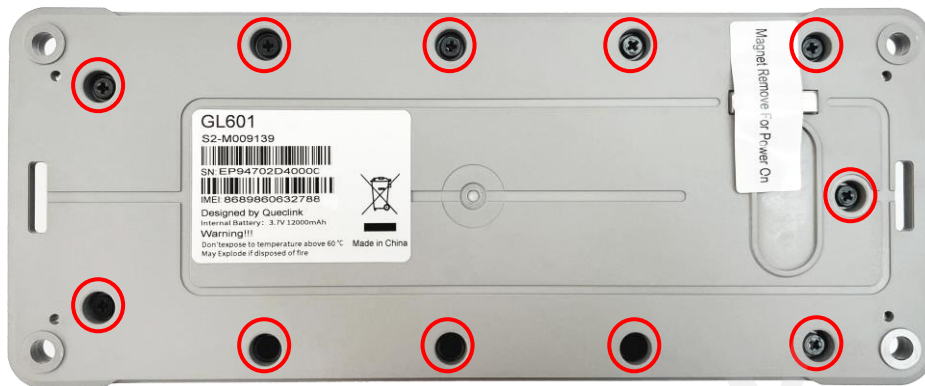
Figure 4. GL601 Series Screw Position
