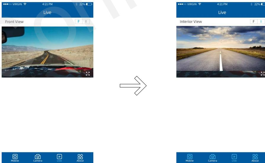
Open the Live window, tap “Front/Interior” button to switch the video source. Adjust the angle of front and interior for best view at first installation.
