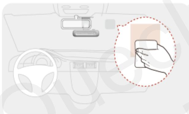
2. Peel off the protective film from the double-sided tape and attach the interior camera to the windshield.
