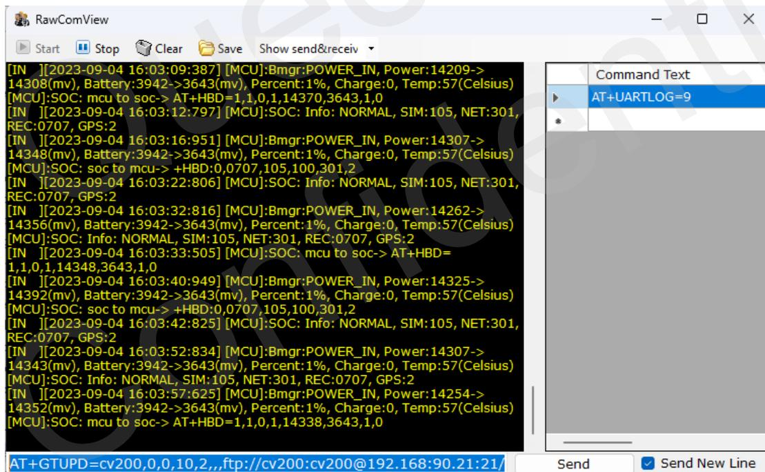
5) Monitor the report feedback on the server or debug window of Manage tool, the local Power indicator is fast flashing during updating. The updating is completed after hear the beep sound.
