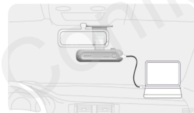
\*Need to install the cable driver probably for USB\_COM communication
