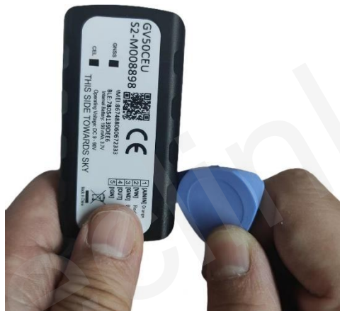
Figure 3: Open the Case
