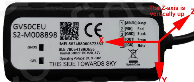
Figure 7: Motion Sensor Direction
