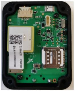
**4** To turn on the device, you can turn on the battery switch or long press the key button for more than 3 seconds.
