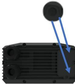
**Step 2:** Insert the SIM card according to the direction indicated by the SIM card slot (the left side of the slot is for the secondary card, and the right side is for the main card).
