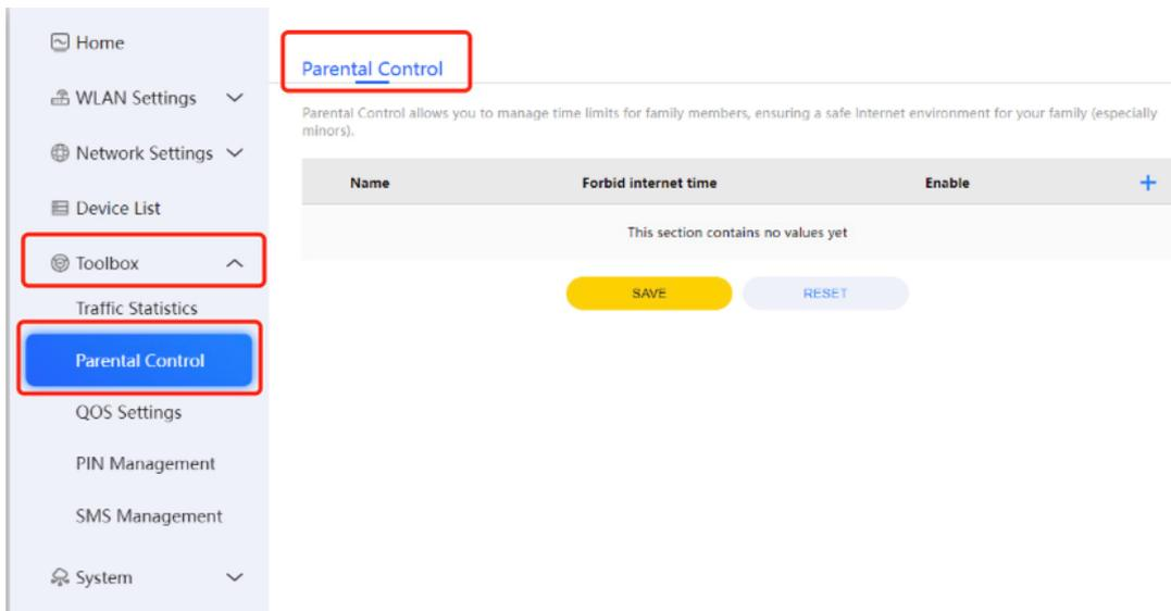
The configuration for child internet protection includes setting a name, selecting the Source MAC address, and defining the times for enabling and disabling the protection.
