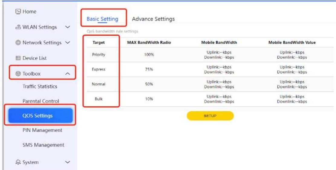
The QoS (Quality of Service) function allows you to limit the bandwidth for mobile networks connections. When the bandwidth policy is enabled and no settings are configured in the advanced settings, the default bandwidth limitation policy for connected terminal devices is set to "Normal".
