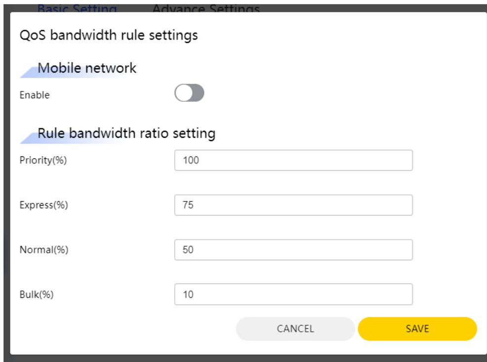
Select “Toolbox”- “QoS Settings”- “Advanced Settings”. QoS Advance Settings allows users to finely tune the QoS by configuring MAC or IP QoS settings. This feature enables users to prioritize specific devices or IP addresses, ensuring a more optimized and efficient network experience based on users' preferences.
