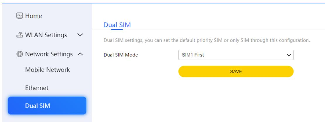
**SIM1 First:** The device will prioritize using the SIM1 network. When the SIM1 network is unavailable or unstable, it will automatically switch to using the SIM2 connection.
