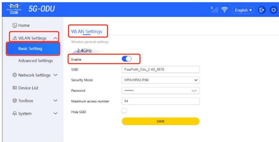
Input SSID, Password, Maximum access number. For Security Mode, there are “OPEN”, “WPA2-PSK” and “WPA/WPA2-PSK” Mode.
