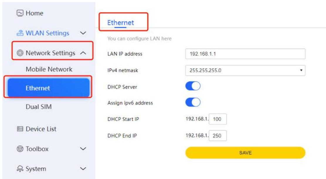
Ethernet Configuration encompasses the IPv4 netmask option, allowing users to define and customize the subnet mask for their network. This feature provides flexibility in tailoring the network layout and optimizing IP address allocation, contributing to a well-organized and efficient networking environment.
