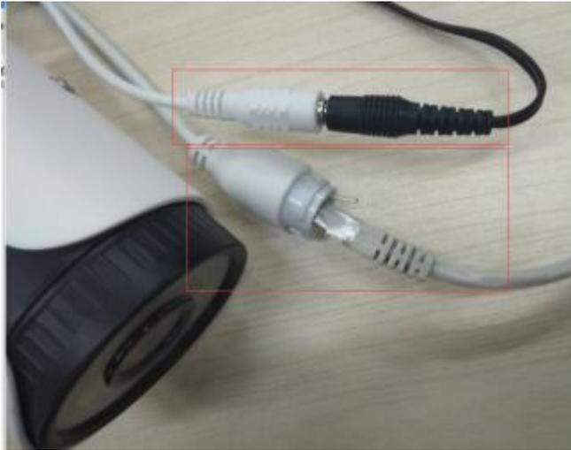
2. POE Powered: Directly powered through the network cable (standard POE 48V power).
