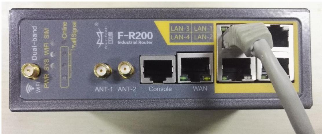
Insert the RJ45 end of the console cable into the RJ45 outlet with sign “console”, and insert the DB9F end of the console cable into the RS232 serial interface of user’s device.
